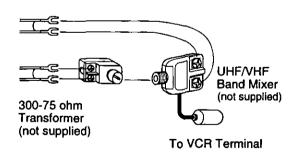
If your TV has both post and plug-type VHF terminals, the post connection is recommended to minimize signal loss.
